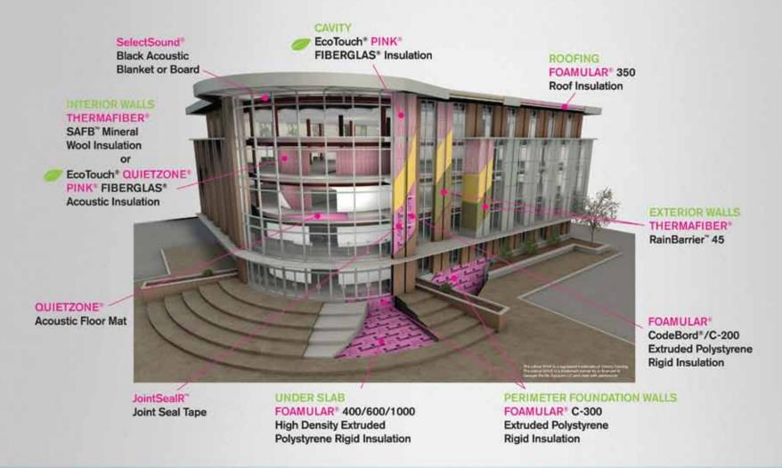
Using Owens Corning EcoTouch® PINK® FIBERGLAS® Insulation, FOAMULAR® Rigid Foam Insulation and Thermafiber® Mineral Wool Insulation helps provide a durable, energy efficient building enclosure. Look to Owens Corning products for energy efficient, acoustically sound and cost efficient solutions in institutional, commercial and industrial buildings.
